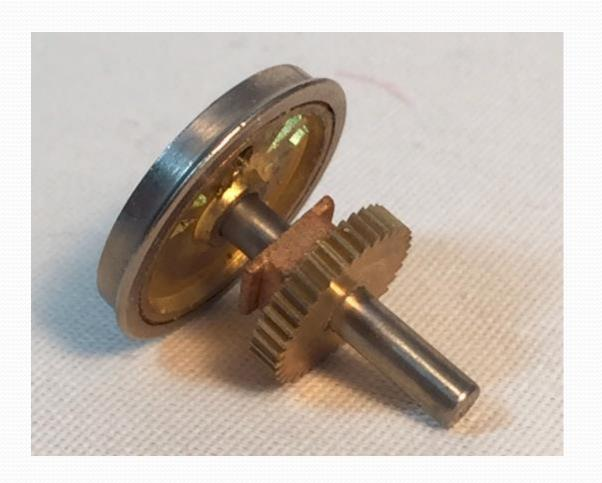
Now re-install the driver on the shaft, lining up the match mark you scribed on the driver and axle earlier.
